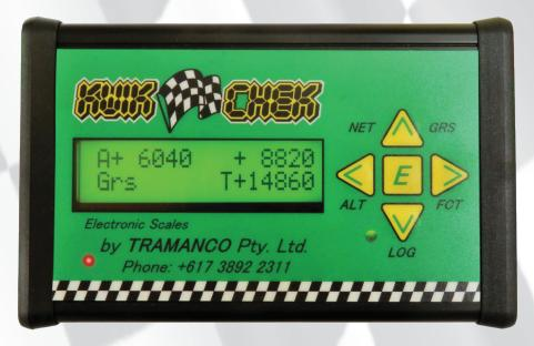
The KWIK-CHEK® 5500 cab mounted unit is a Kwik Weigh to obtain the weights of single axles or groups of axles.
